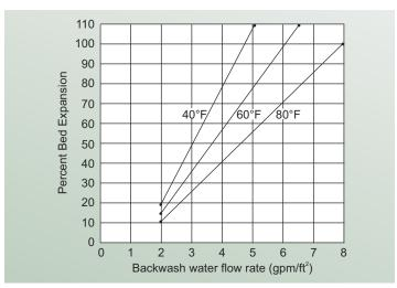
Fig. 2 Bed Expansion vs. Backwash Flow Rate at various degrees Fahrenheit (F°)
