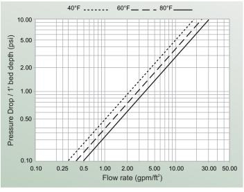
Fig. 1 Pressure Drop vs Flow Rate at various degrees Fahrenheit (F $^{\circ}$ )
