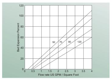
Fig. 2 Bed Expansion vs Flow Rate at various degrees Fahrenheit (F $^{\circ}$ )
